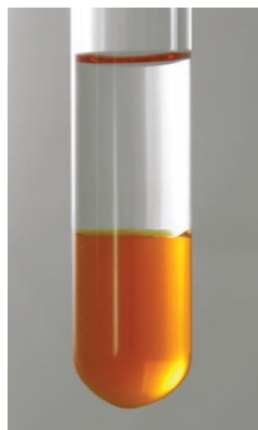
Figure 1. Two-phase system composed of n -hexane and PC with [\text{Ir}(\text{cod})(\mathbf{4})]\text{BAR}^{\text{F}}_4 .
